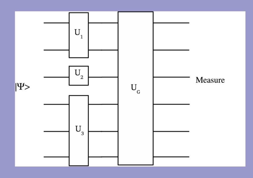
The quantum circuit that exemplifies the operational meaning of the Groverian entanglement measure for a pure quantum state with arbitrary partitioning.
