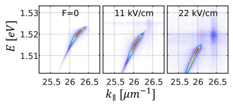
Measured dispersion under three different fields. *The exciton and the entire polariton branch* undergo a redshift as the field intensity grows.
