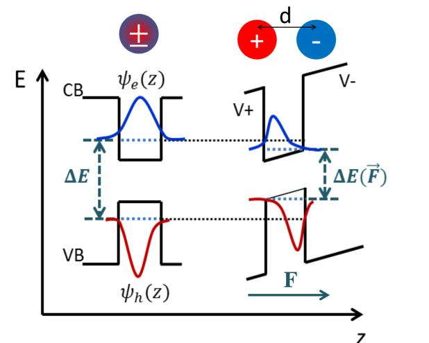
Illustration of the QW potential and the exciton dipole, with and without electric field.
