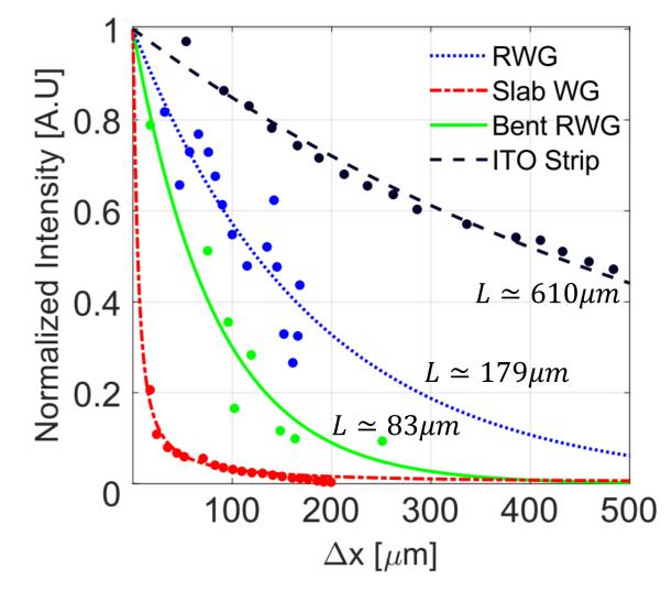
*Compression of the propagation distance in* the different geometries.
