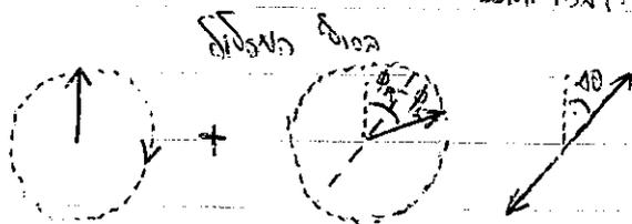
$$\Delta\theta = \frac{1}{2} \int_0^d (K_R - K_L) ds = \frac{1}{2} \int_0^d \frac{\omega_p^2 \omega_c}{c \omega^2} ds = \dots$$
