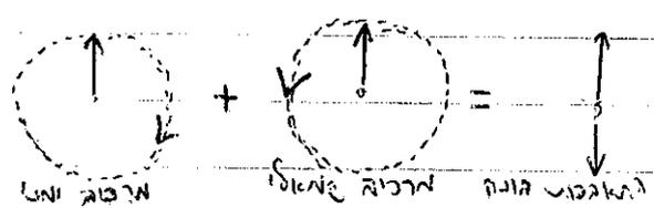
$$K_{RL} = \frac{\omega}{c} \sqrt{1 - \frac{\omega_p^2/\omega^2}{1 + \frac{\omega_c}{\omega}}} \approx \frac{\omega}{c} \sqrt{1 - \frac{\omega_p^2}{\omega^2} \left(1 \pm \frac{\omega_c}{\omega}\right)}$$
