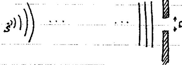
The EM field of the wave causes the charges on the screen to move. They in turn produce electric and magnetic fields that should be added to the incident wave in order to find the total EM field. This is a difficult task and we're going to make few approximations.
