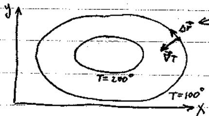
Consider the infinitesimal vector  $\Delta\vec{r}$  connecting two neighboring points on an equi-temperature curve. Since  $\Delta T = \vec{\nabla}T \cdot \Delta\vec{r} = 0$  between the two points
