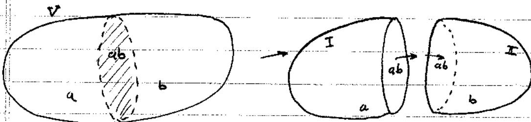
The flux of a vector field from volume I = flux through a + flux through ab
