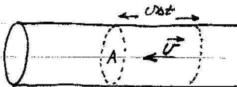
It is clear that during the time  $\Delta t$  all the particles that are at a distance  $v\Delta t$  or less from  $A$  will cross it.
