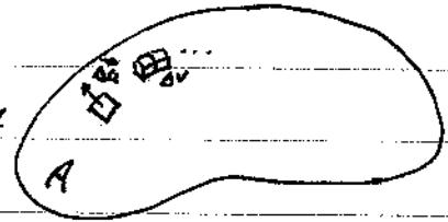
$$\text{Flux of } \vec{J} \text{ through } A = \sum_i \vec{J}_i \cdot \Delta \vec{a}$$
