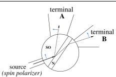
FIG. 4 (color). A spin transistor. A spin current at terminals A and B is controlled by modulation of the magnitude of  $\alpha$ .
