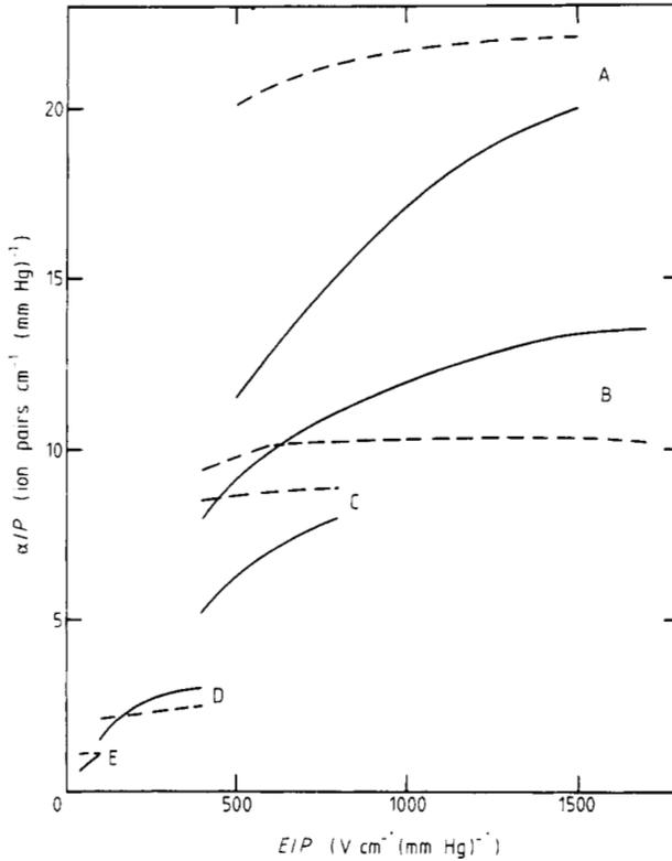
**Figure 1.** First Townsend ionisation coefficient. A, Hg; B, Ar; C, N<sub>2</sub>; D, Ne; E, He. Broken curves, calculations; full curves, experimental results.
