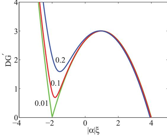
FIG. 4. (Color online) Stability function  $DG'$  versus  $|\alpha|\xi$  for  $\alpha > 0$  and different values of initial signal amplitude  $B_{30}$ .  $DG' \gg |\alpha|$  is required for continuing autoresonance in the system.  $B_{30} = 0.2$  for the upper blue curve,  $B_{30} = 0.1$  for the intermediate red curve and  $B_{30} = 0.01$  for the lower green curve.
