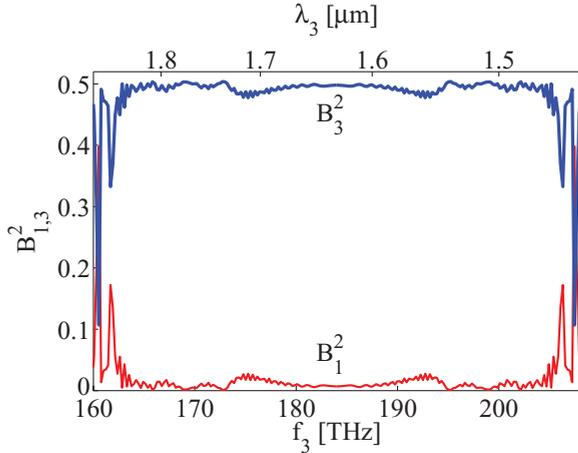
FIG. 6. (Color online) The amplification spectrum of the autoresonant OPA. The normalized intensity of the signal,  $B_3^2$  (blue upper line), and the pump,  $B_1^2$  (red lower line), versus the signal frequency  $f_3$  and wavelength  $\lambda_3$ .
