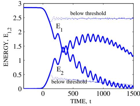
**Figure 2.** Autoresonant evolution of the energies  $E_{1,2}$  of the two coupled oscillators in system (18). The evolution just below the threshold for capture into resonance is shown by dotted lines.
