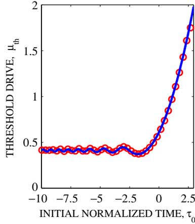
**Figure 1.** Threshold for autoresonance in the nonlinear Schrödinger equation (7) versus initial normalized time  $\tau_0$  (solid line). The circles show a similar threshold for the normalized coupling parameter in the two coupled oscillators system (18).
