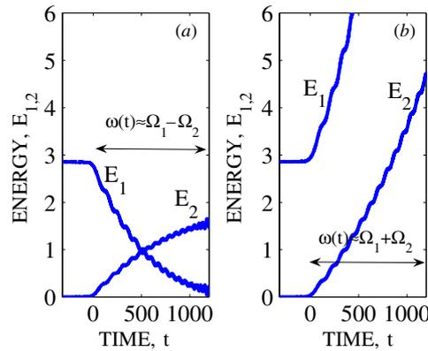
**Figure 3.** The energies  $E_{1,2}$  of the coupled oscillators in system (18) with an oscillating coupling parameter. (a) Passage through  $\Omega_1 - \Omega_2$  resonance; (b) passage through  $\Omega_1 + \Omega_2$  resonance. The autoresonant decrease or increase of the energy of the initially excited oscillator 1 is obtained by choosing one of the resonances.
