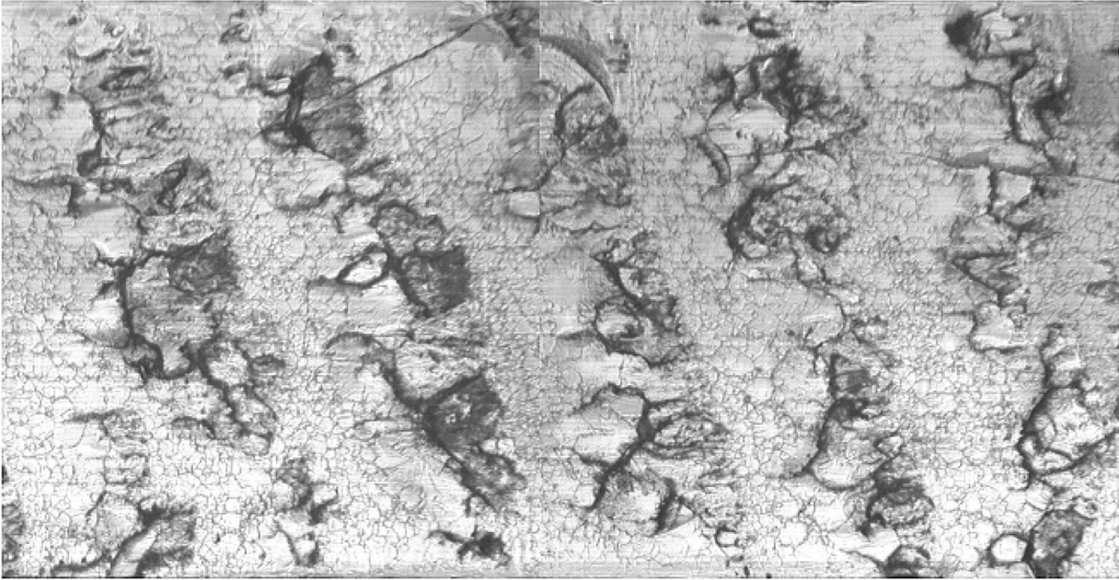
Fig. 16. A photograph of typical rib-like patterns observed on the fracture surface of PMMA. The distance between ribs is approximately 1 mm. On smaller scales parabolic markings can be discerned.
