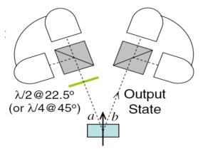
■  $a_H^{\dagger}$ ,  $a_V^{\dagger}$  modes bunch when rotated to 45° linear or right-left circular polarizations → No coincidence
