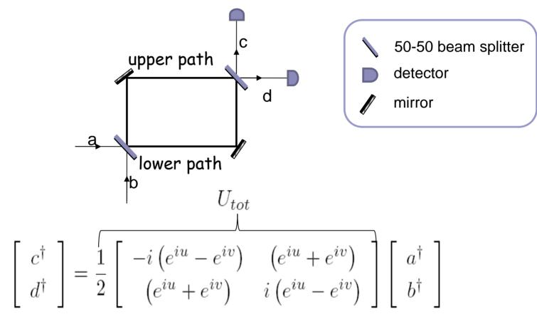
The phase to be measured:  $\Phi = \vec{k} \cdot l_{upper} - \vec{k} \cdot l_{lower}$
