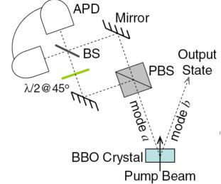
Input state (PDC):  $|\psi_{2}^{-}\rangle = \frac{1}{\sqrt{3}}(|2,0\rangle_{a}|0,2\rangle_{b} - |1,1\rangle_{a}|1,1\rangle_{b} + |0,2\rangle_{a}|2,0\rangle_{b})$
