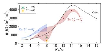
FIG. 20. B(E2) values in  $e^2 \text{fm}^4$  for  $2_B^+ \to 0_B^+$  in Zr isotopes and  $2_1^+ \to 0_1^+$  in Xe isotopes, as a function of  $N_\pi N_\nu$ . Shown are calculated values (black dots connected by a line) and experimental values (blue and red dots) with errors in shaded areas. For  ${}^{98}\text{Zr}$  ( $N_\pi N_\nu = 8$ ), the experimental upper and lower limits are from [29,31] and the explicit values,  $\blacktriangle$  and  $\spadesuit$ , are from [32] and [33], respectively.
